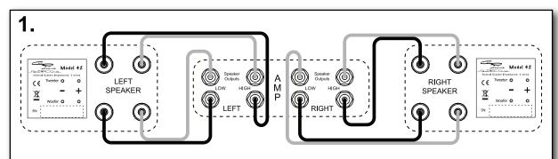
Connect both the right and left speakers to the amplifier as shown. Failure to do this correctly will result in audio degradation. High output to tweeter - low output to woofer - red to red - black to black.
